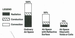
As indicated here, heat transfer by convection is a major consideration, which can be almost eliminated by the use of insulation material, such as EPS.
